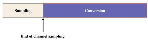
→As soon as the sampling is completed it is possible to prepare next conversion (for instance switching I/Os) during the conversion phase.
